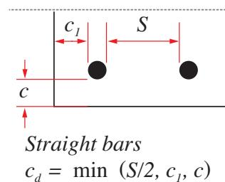
Note: Equation A is valid for cracked and uncracked concrete if no additional requirement is provided in product ETA.
